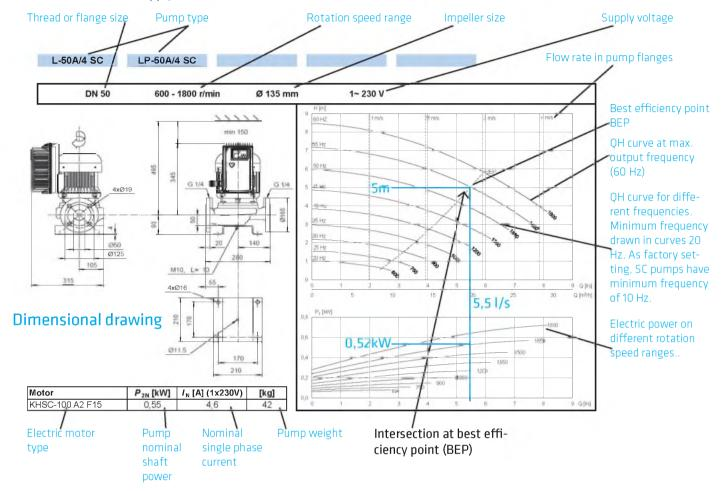
**NOTE!** Liquid density and viscosity affect the amount of power required. Please check that the motor power is sufficient for liquids with a higher density and viscosity than water. Please contact Kolmeks for further information.
