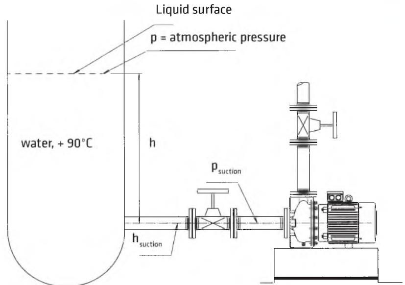
**Example 2:** Open tank ( $p = \text{atmospheric pressure} = 10 \text{ m}$ ) where water temperature is at the maximum  $+ 60^\circ\text{C}$  ( $p_h = 2 \text{ m}$ ), suction pipe pressure losses  $1 \text{ m}$ . Pump duty point  $14 \text{ l/s}$ ,  $50 \text{ m}$ . Pump  $\text{NPSH}_{re} = 3.1 \text{ m}$ . QUESTION: At which level in relation to the surface of the liquid should the pump be installed?
