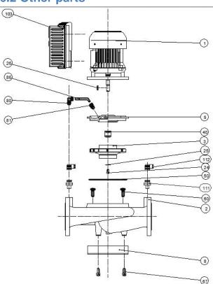
1 Electric motor 2 Pump housing 3 Impeller **5** Sealing flange 8 Foot (not always) 24 VSrew or nut 25 Washer 26 Key 40 Shaft seal 50 O-ring or gasket 60 VSrew or nut 67 VSrew 80 Pipe union (L- and ALH -serie) 81 Pipe union (L- and ALH -serie) 86 Cooling pipe (L- and ALH -serie) **103 Frequency converter** 111 Transmitter quick connector(VSB, VSC, VSD) 112 Transmitter(s) for pressure, pressure difference or temperature (VSB, VSC, VSD, VSF)
